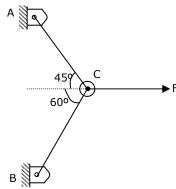
48. The maximum force F in kN that can be applied at C such that the axial stress in any of the truss members DOES NOT exceed 100MPa is
