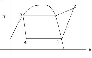
Power required for compressor =  $m_r (h_2 - h_1)$
