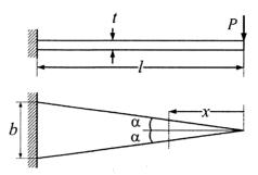
Q.52 The area moment of inertia about the neutral axis of a cross-section at a distance x measured from the free end is
