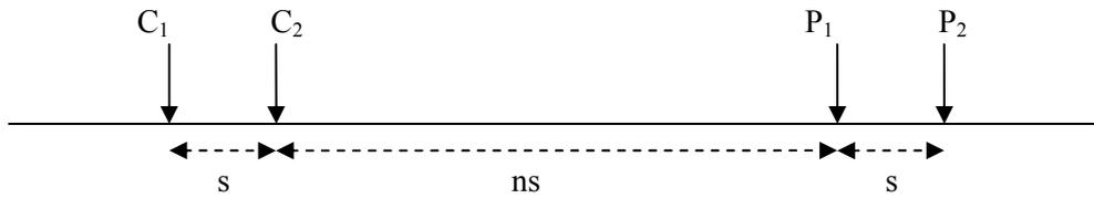
Q.54 The geometrical factor for the above axial dipole array is
