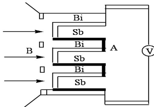
Description: A thermopile consists of thermocouples connected in series which are in turn connected to a galvanometer. One set of junctions (Sb) is blackened and other set of junctions are protected from heat.
