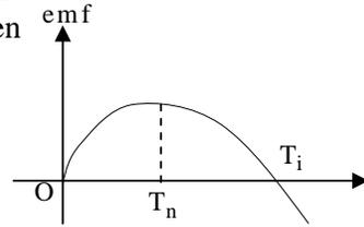
Then  $e = aT + bT^2$ , which is parabolic in nature.
