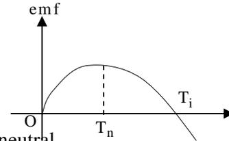
Beyond the temperature of inversion the thermo e.m.f. reverses its direction. The temperature of inversion depends upon the temperature of cold junction.
