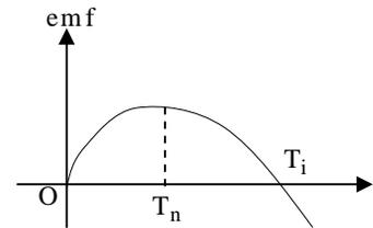
Inversion Temperature ( $T_i$ ): The temperature of the hot junction at which the direction of thermo emf is reversed in a thermo couple is called inversion temperature.  $T_i = -\frac{a}{b}$
