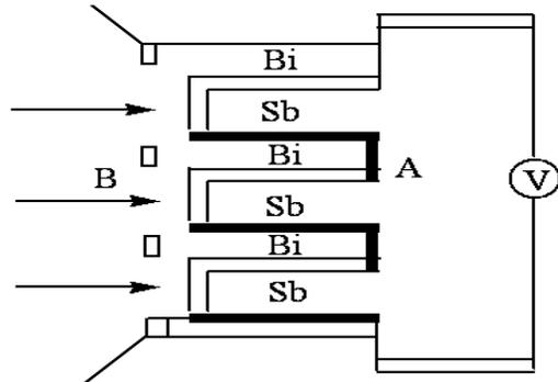
One set of the end A, is covered with a brass cap to maintain the temperature of these junctions constant. The junctions on other side 'B' are coated with lamp black and exposed to heat radiation.
