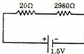
$\therefore$  Potential difference across the potentiometer wire =  $\frac{1}{150}(1.5) = \frac{1}{100}V$
