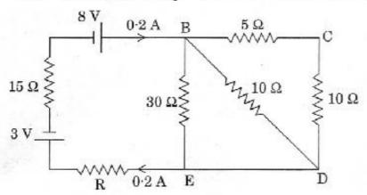
Calculate the value of the resistance R in the circuit shown in the figure so that the current in the circuit is 0.2 A. What would be the potential difference between points B and E?
