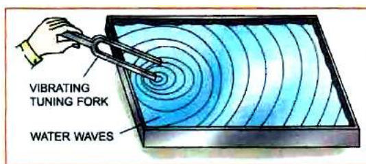
The vibrating prongs of the tuning fork produce circular waves in water
